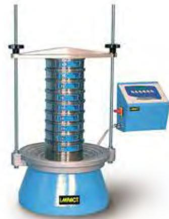
The shaker can hold up to 10 sieves. It is fitted with a digital 1 to 999 minute timer, accessed through the digital control panel. This separate panel also gives the user control of the vibration intensity and pauses between sieving actions, which is particularly useful when sieving fine materials.
